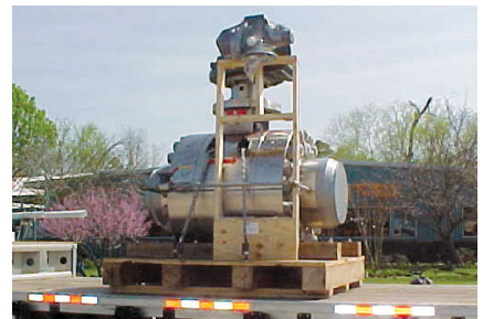
This large bore 24-inch metal seated ball valve was one of several chosen for a tar sands upgrade project. Ability to meet the stringent deadline was crucial to the success of the start-up.
